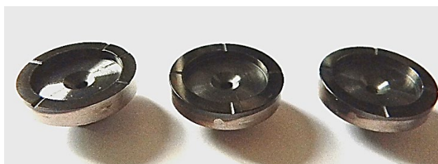
Fig. 2. IM125 titanium samples with CN_x coating for tribological testing.
